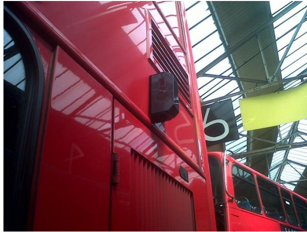
Figure 12: Rear-mounted nearside camera system (rectangular box mounted to outside of bus)
