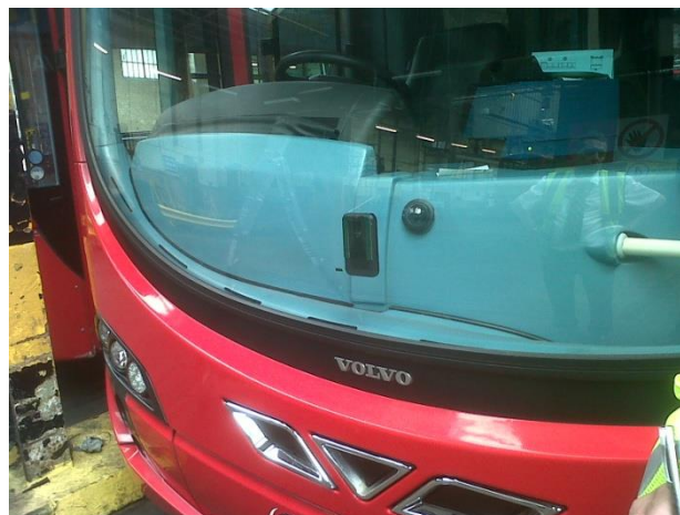
Figure 11: Front camera system (rectangular box in the windscreen)
