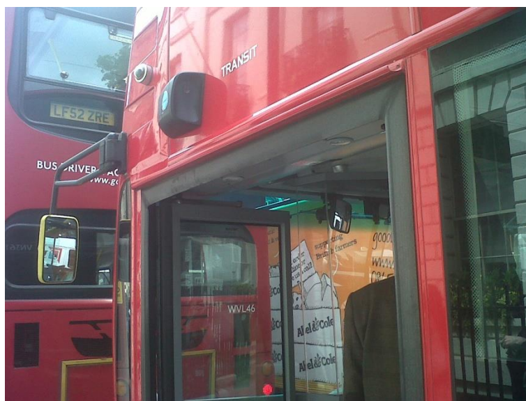
Figure 9: Processing equipment fitted to the nearside front of a London double-decker bus (curved black box fitted above the passenger door)
